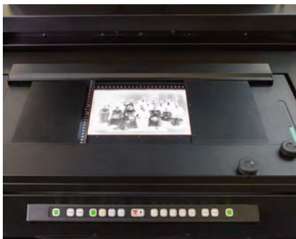
Holder for glass plates, continuously adjustable
